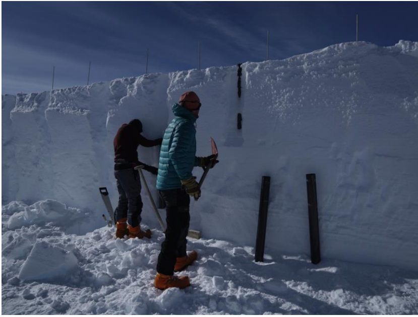
Figure 3: Sampling procedure in the OIR trench. The first carbon fiber tube (liner) is pushed into the snow after excavation of the trench. The positions were marked with a small bamboo pole. After retrieval of the first profile, the vertically consecutive second and third liners were taken. Two empty liners lean at the trench wall. The last liner had to be dug out partly as the trench was only 2 to 2.5 meters deep.
