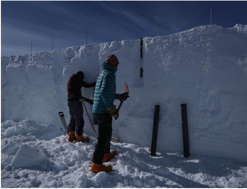
5 Figure 3: Sampling procedure in the OIR trench. The first carbon fiber tube (liner) is pushed into the snow after excavation of the trench. The positions were marked with a small bamboo pole. After retrieval of the first profile, the vertically consecutive second and third liners were taken. Two empty liners lean at the trench wall. The last liner had to be dug out partly as the trench was only 2 to 2.5 meters deep.
