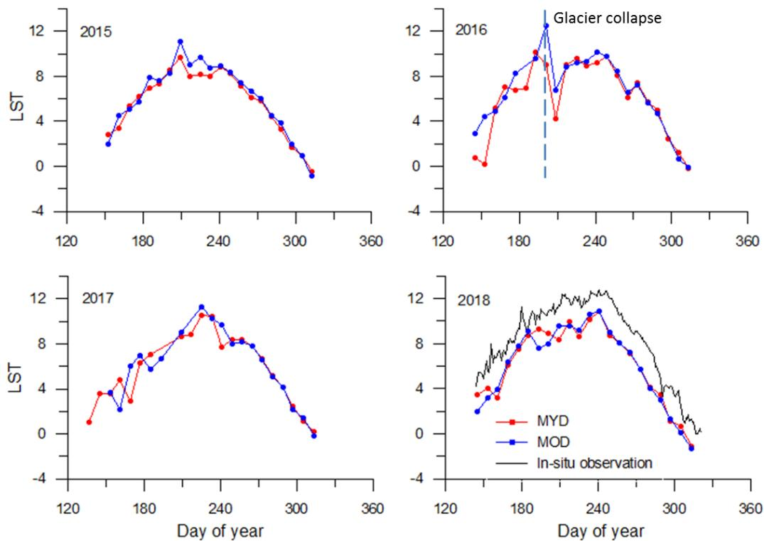
580 **Figure 8: Time series of lake surface temperature (LST) derived from MYD11A2 (red cycles) and MOD11A2 (blue cycles) at Memar Co between 2015 and 2018. The thin line represents in-situ lake water temperature at the shoreline. The dashed line in 2016 is the time of the first glacier collapse.**
