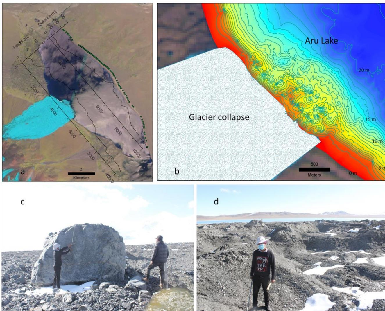
525 **Figure 4:** a: The extent of the first glacier collapse (Sentinel-2 image on 21 July, 2016) and the impact wave at the opposite shore of Aru Co (green dots). b: The uneven lake bathymetry at Aru Co near the first glacier collapse. c, d: A large amount of debris left after the fragmented ice mass melting (photos taken on 3 October, 2019 by Yanbin Lei).
