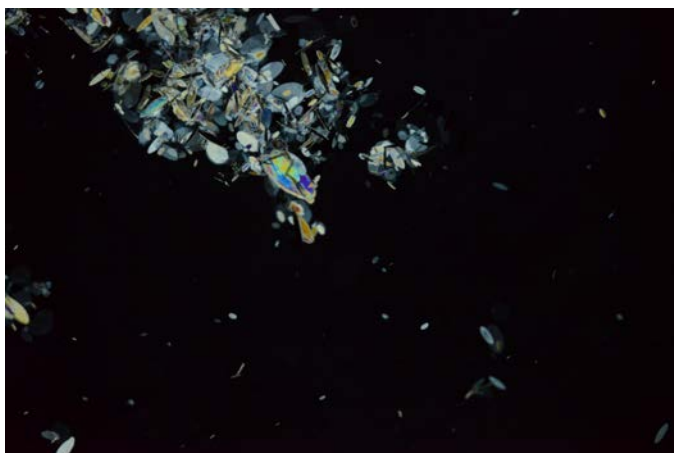
Figure 4: Raw digital images showing frazil particles and flocs for a) 35 %, and b) freshwater. Image dimensions are 3.07 cm by 4.61 cm.
