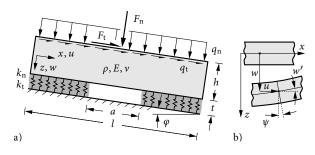
**Figure 2.** Snowpack modeled a) as a beam on elastic foundation of infinite set of shear and compressive springs b) using Timoshenko beam kinematics.
