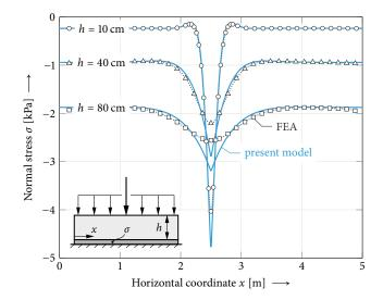
**Figure 7.** Bridging effect evident in weak layer normal stresses depending on the slab thickness. Peak stresses and the width of the skier loaded snow pack changes with different slab thicknesses. Model results (solid lines) are compared against the reference solution (markers  $\bigcirc, \triangle, \square$ ). Model parameters are chosen as given in Table 1.
