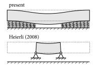
**Figure 12.** Impact of model assumptions on slab deformations. Heierli (2008) considers only the unsupported section of the slab and, hence, does not account for deformations of the beam segment resting on the intact weak layer, which contributes to the total stored energy.
