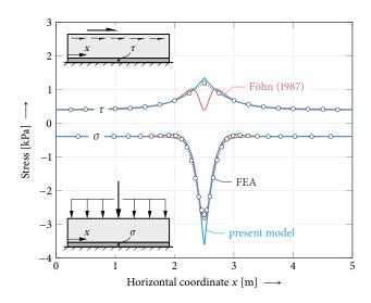
**Figure 6.** Normal and shear stresses owing to pure vertical and pure horizontal combined skier and slab weight loading, respectively. Comparison of present model (blue) and Föhn (1987) model (red) to FEA results (circles). Model parameters other than h = 20 cm, t = 1 cm,  $E_{\text{slab}} = 5$  MPa,  $E_{\text{weak}} = 0.15$  MPa and  $\rho = 200$  kg m<sup>-3</sup> are chosen as given in Table 1.
