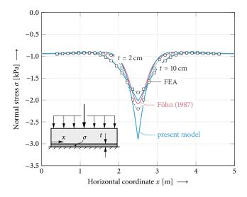
**Figure 8.** Effect of the weak layer thickness on local weak layer normal stresses. The weak layer thickness changes the size of the skier load affected part of the weak layer and also the peak value of the stress. Thicker, more compliant weak layers distribute the load on a larger area and lead to lower peak stresses. Model results (solid lines) are compared against the reference solution (markers  $\bigcirc, \square$ ). Model parameters are chosen as given in Table 1.
