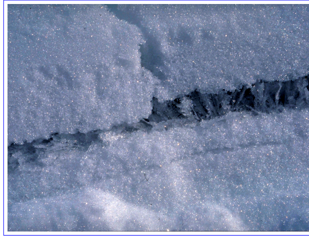
Figure 1. Weak layer of buried surface hoar. Left of the vertical slab fracture the weak layer has collapsed, whereas on the right hand side the porous weak layer is still intact. Reprinted from the Journal of Glaciology (Jamieson and Schweizer, 2000) with permission of the International Glaciological Society.
