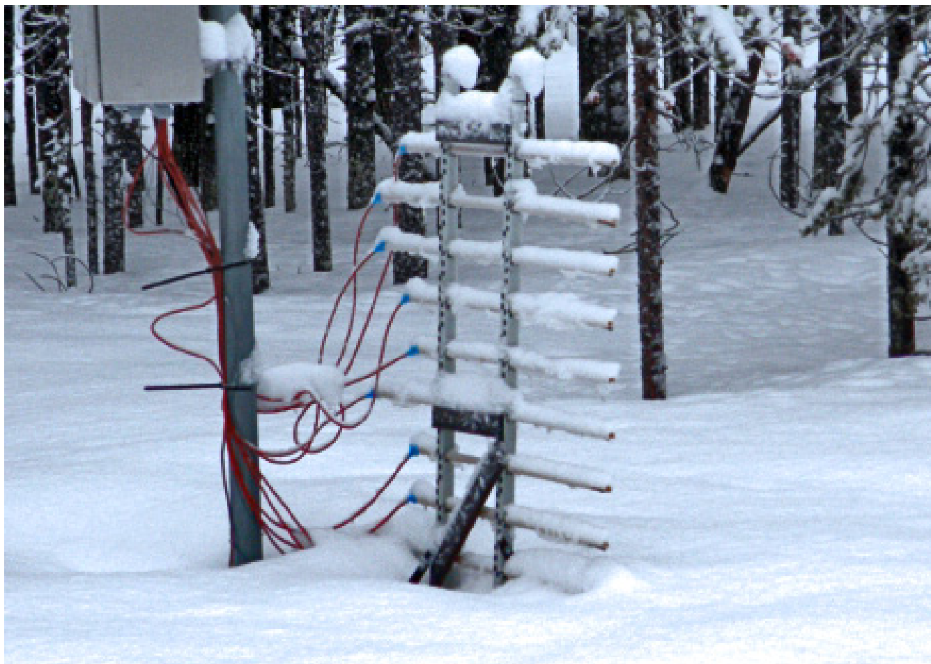
Figure 3. Snow temperature was measured at every 10 cm height by an array of horizontally oriented temperature sensors at the meteorological mast.
