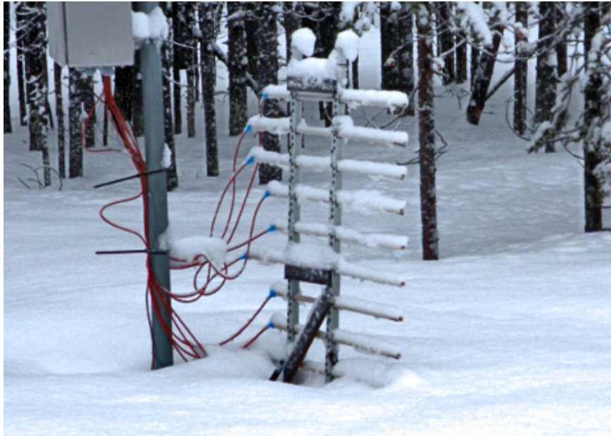
Figure 4. Snow temperature was measured with an array of horizontally oriented temperature sensors at the meteorological mast.
