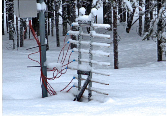
Figure 4. Snow temperature was measured at every height by with an array of horizontally oriented temperature sensors at the meteorological mast.
