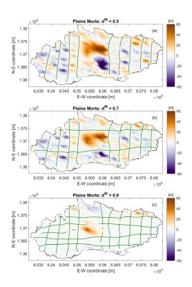
Figure 9: Plaine Morte model misfit h<sup>true</sup> - h<sup>est</sup> after selected stages of the experimental design procedure using observed data (see also vertical dashed lines in Figure 7). The selected GPR profiles are superimposed with green lines.
