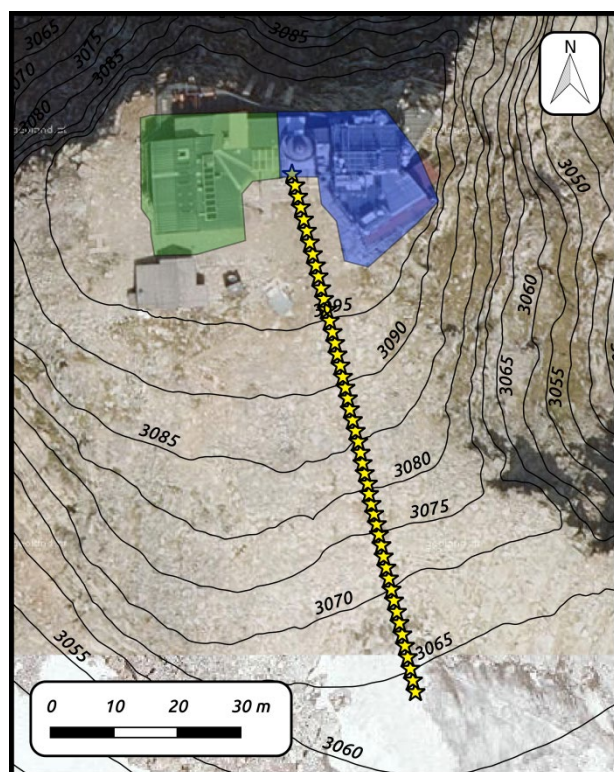
Figure 3: Detailed view of the study area with the Sonnblick Observatory (blue) and the hut of the Austrian Alpine Association (green) on top of the summit of Hoher Sonnblick. The location of the profile for the refraction seismic measurements conducted in May 2017 is indicated by the shot positions (yellow stars; shot positions correspond to geophone positions).
