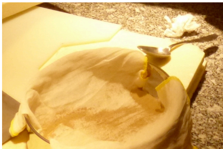
Figure 1: Sieve with textile mesh used to spread dust on the snow surface (the spoon gives the scale)
