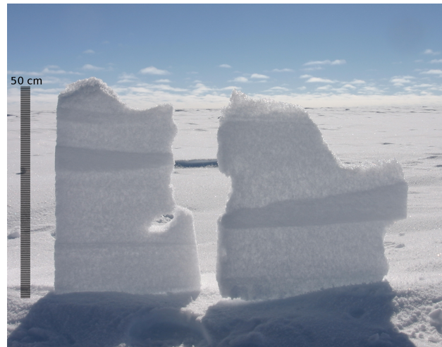
Figure 15. Photograph of a thin vertical section extracted from 5 m depth at Dome C in January 2010 showing the persistence of heterogeneity at depth.
