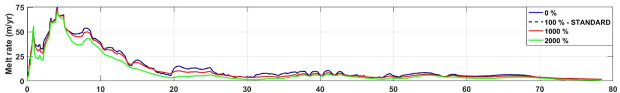
Figure S5: Sensitivity of the submarine melt rate along the centreline of the 79NG ice tongue due to the tidal flow in the cavity. The tidal velocity in the STANDARD case is 1.18 cm/s. Note that this are results from Anhaus, 2017 (Master thesis, unpublished) and here the STANDARD case has tides of 1.18 cm/s and a subglacial discharge of  $1 \times 10^{-03} \text{ m}^2/\text{s}$ .
