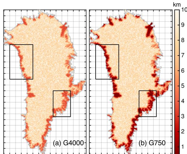
**Figure 2.** Horizontal mesh resolution (in km) used for G750 (a) and G4000 (b). Data are clipped at 0.5 and 10 km. The horizontal resolution of a triangle is defined by its minimum edge length. The grey line delineates the initial ice domain. Grey grid lines indicate 100 km. The black boxes indicate the northwestern and southeast subsets used in following figures.
