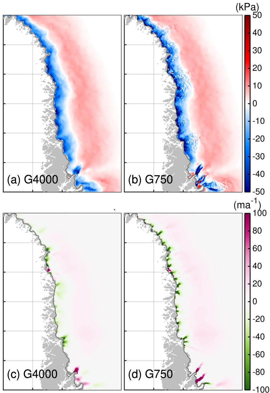
**Figure 13.** (a,b) Difference of driving stress between 2100 and 2015 for the northwestern region. (c,d) Difference of basal velocity between 2100 and 2015 for the northwestern region. Region subsets are shown in [See-Fig. 2](#). Dark gray line indicates the initial ice extent. Thin black line indicating the grounding line is not visible as it falls together with the calving front. The grey silhouette shows the Greenland land mask from BedMachine v3.
