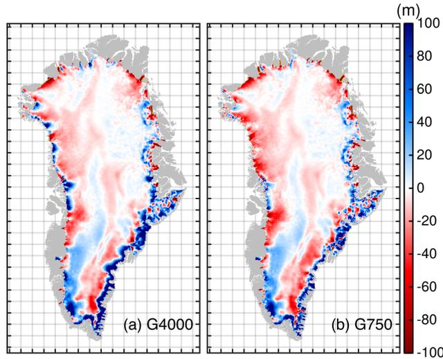
**Figure 7.** Difference of ice thickness between 2100 and 2015 for the ctrl run. (a) G750 simulation and (b) G4000 simulation. The grey silhouette shows the Greenland land mask from BedMachine v3. Positive values represents thickening, and negative shows thinning. Thin yellow line show the grounding line at the year 2100.
