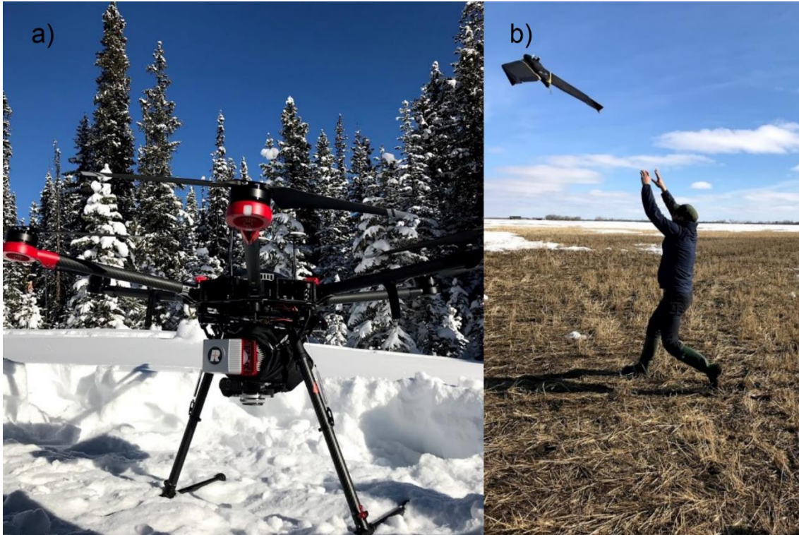
Figure 2: UAV-lidar platform: Riegl miniVUX1-UAV mounted on DJI M600 Pro (a) and UAV-SfM platform: Sensefly EbeeX (b).
