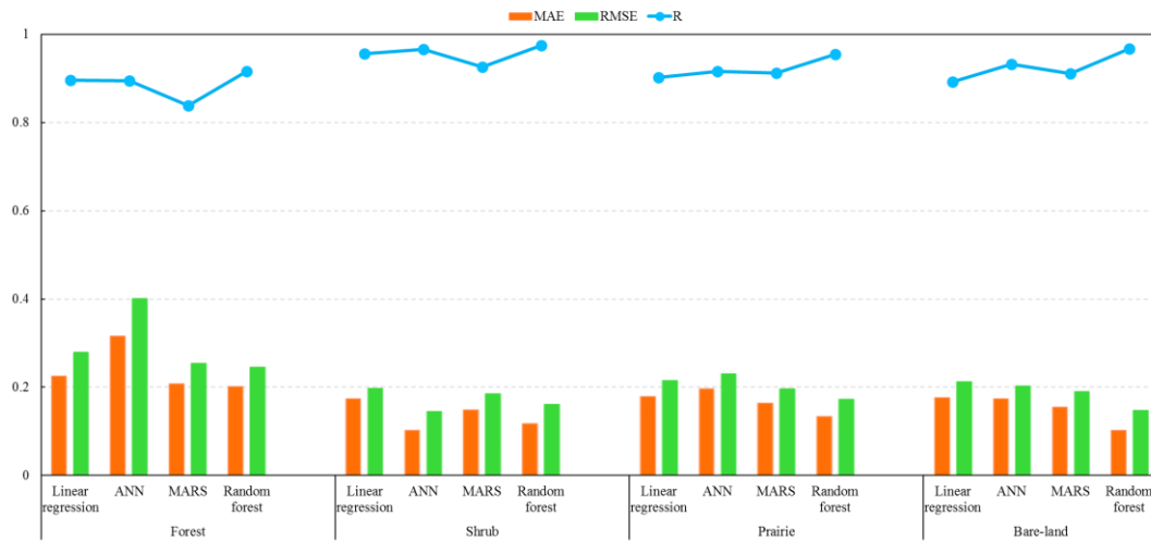
5 Fig. 5. The variation of the accuracy indexes (MAE, RMSE and R) on four algorithms (linear regression, ANN, MARS and Random forest) for four land cover.
