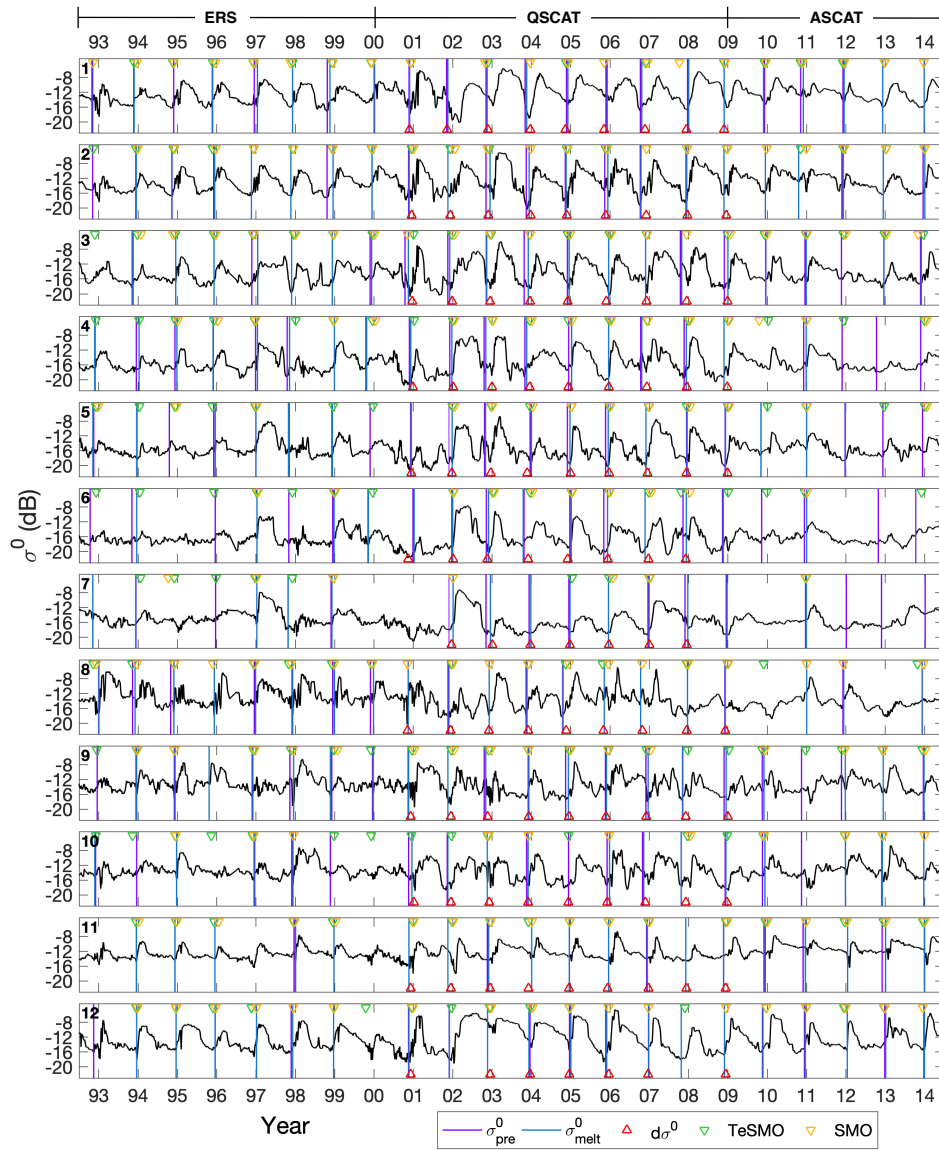
Figure 2. Time series of 6-day mean backscatter coefficients ( \sigma^0 ) from 1992/1993 to 2014/2015 averaged over the respective 9 pixels at the study locations on perennial sea ice (Figure 1, 1-12). Purple and blue lines show the scatterometer-derived snow pre-melt ( \sigma^0_{\text{pre}} ) and melt ( \sigma^0_{\text{melt}} ) onset dates when the algorithm criteria were met (Section 2.2.1). Red triangles indicate the snowmelt onset retrieved from diurnal backscatter variations ( d\sigma^0 ) of QSCAT data. Green and yellow triangles show the Temporary Snowmelt Onset (TeSMO) and Continuous Snowmelt Onset (SMO) derived from passive microwave observations from Arndt et al. (2016).
