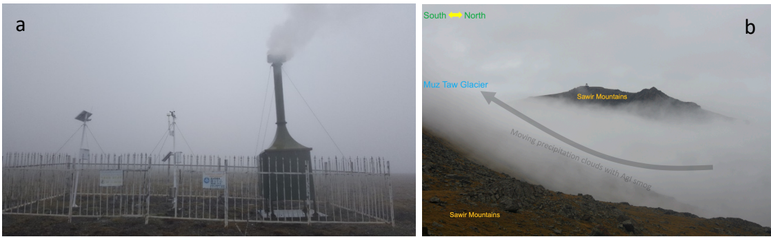
Figure 3 a) Igniting the AgI smog generators along the terminal river when the cloud accumulated late on the afternoon of 19 and 22 Aug 2018, and b) the accumulating of clouds in the valley of the Muz Taw Glacier favoured by the AgI particles moved up towards the summit of the glacier.
