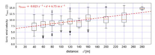
Figure 7: Sonic anemometer wind velocity as a function of the transport distance of the blowing snow events for evaluation period one and two.
