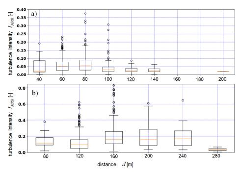
Figure 8: Turbulence intensity determined from the MRR spectral width of the Doppler spectrum of the range gate defining the blowing snow transport distance (Fig. 3) as a function of transport distance for evaluation period a) one, and b) two.
