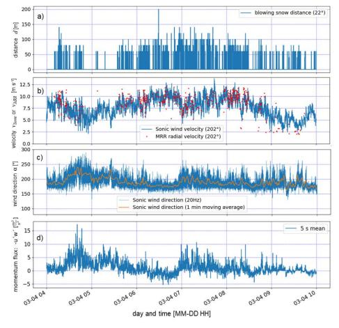
Figure 4: a) Temporal evolution of the horizontal transport distance of all blowing snow events of evaluation period one (2019-03-04, 0400 UTC+1 – 1000 UTC+1). b) Wind velocity parallel to the MRR direction (202 $^{\circ}$ ) measured with a sonic anemometer compared to the close range (20 - 40m) blowing snow radial velocities measured with the MRR (see Fig. 3a). c) Wind direction (mainly 180 $^{\circ}$  - 220 $^{\circ}$ ) and d) momentum flux –u'w' calculated using the sonic anemometer data.
