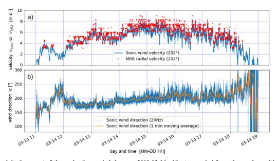
Figure 9: Precipitation event of the evaluation period three on 2019-03-14 with strong wind from the south resulting in blowing snow and preferential deposition north of the Snow Drift Station as shown in Fig. 2. a) Sonic anemometer wind velocity and MRR radial velocity, and b) wind direction (similar as in Fig. 4b and c)
