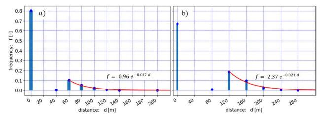
Figure 6: Histogram of the transport distance of all blowing snow events for evaluation period a) one (Fig. 4a), and b) two, including an exponential fit for distances larger than the minimal transport distance.
