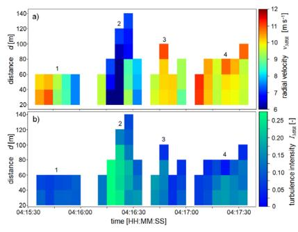
Figure 3: a) MRR radial velocity in the azimuth direction  $22^{\circ}$  for a two-minute period containing four different blowing snow events on 2019-03-04. b) Corresponding turbulence intensity *I*.
