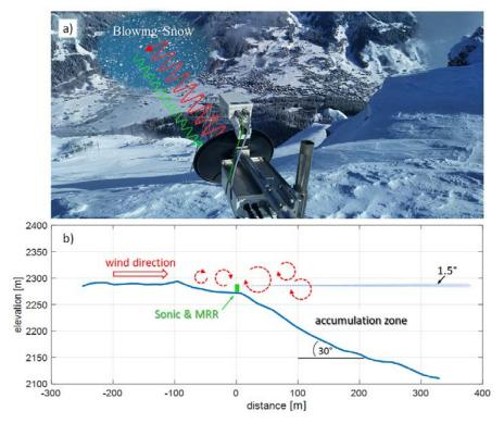
Figure 1: a) Picture of the study site: The Micro Rain Radar (MRR) is looking horizontally from the ridge measuring the radial velocity and distance of blowing snow clouds across the valley. b) Transect of the topography in the viewing direction of the MRR (aspect ratio is 1:1).
