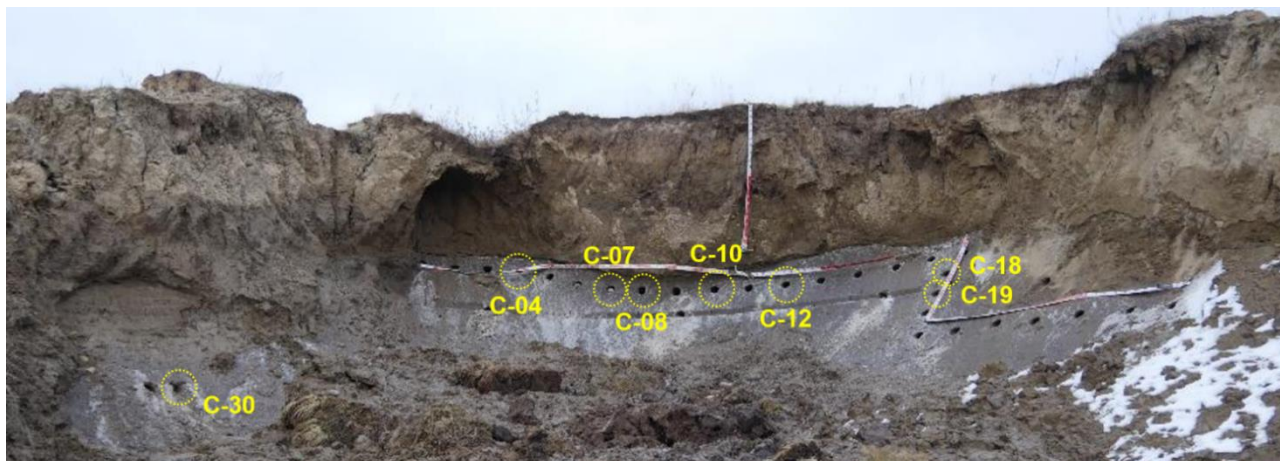
Supplementary Figure 2. Images of ground ice outcrops at Churapcha (central Yakutia) site. Locations of the samples used in this study are indicated by yellow dotted circles.
