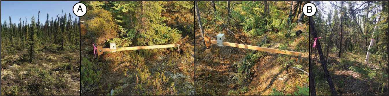
Figure 1. Overview images and close-up photographs of ground cover around tilt arms showing the character of the sites instrumented. Site Evil Peat (A), similar to site Drill the Chill, is in a peatland with open black spruce and tamarack forest. Site Active Slayer (B) is in dense black-spruce forest overlying hummocks in mineral soil.
