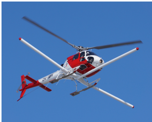
Figure 2. Helicopter in survey configuration. Radar antennas were mounted in the lateral booms, which measure 11.52 m tip-to-tip; the front boom was empty. The laser altimeter and dSLR camera were mounted to the right of the pilot’s seat, using a pre-existing window.
