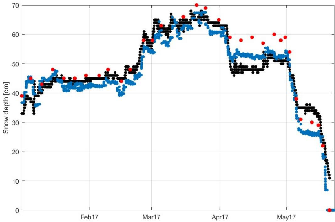
655 **Figure 6.** Sodankylä Peatland: Comparison between visual estimations (red dots), ultrasonic measurements (black dots), FMIPROT estimations (blue dots) in the first half of 2017.
