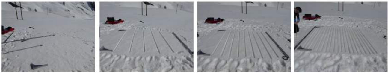
Figure 2. Studied surfaces of experiment A (Table 1), from left to right: A-smooth, A- \eta 7%, A- \eta 13%, and A- \eta 27% sites.
