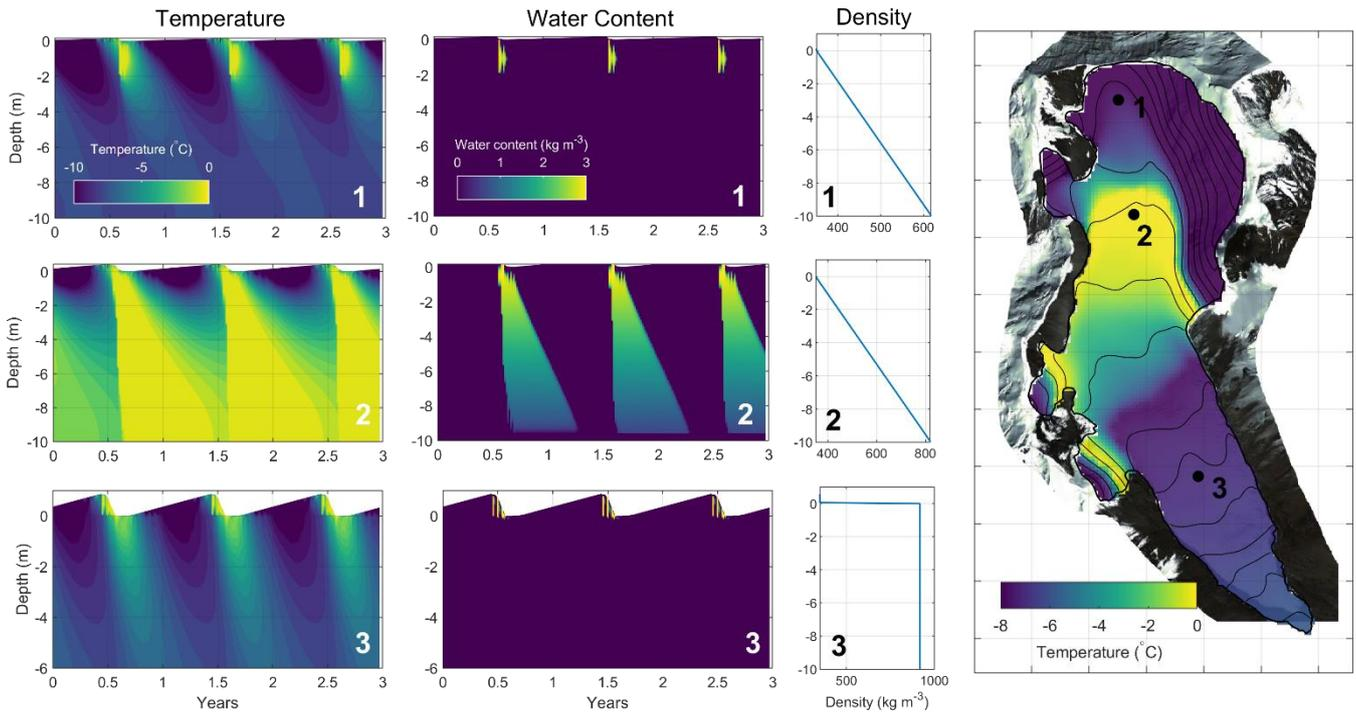
640 **Figure 5. One-dimensional temperature, water content and density modeled in the first 10m-depth during 3 years and at three locations on the glacier. The one-dimensional model is forced by a reference temperature/precipitation annual cycle until reaching a stationary periodic response at 10 m-depth. Mean annual temperature at 10 m-depth is then used as an upper boundary condition for the thermo-mechanical model (mapped on the right panel).**
