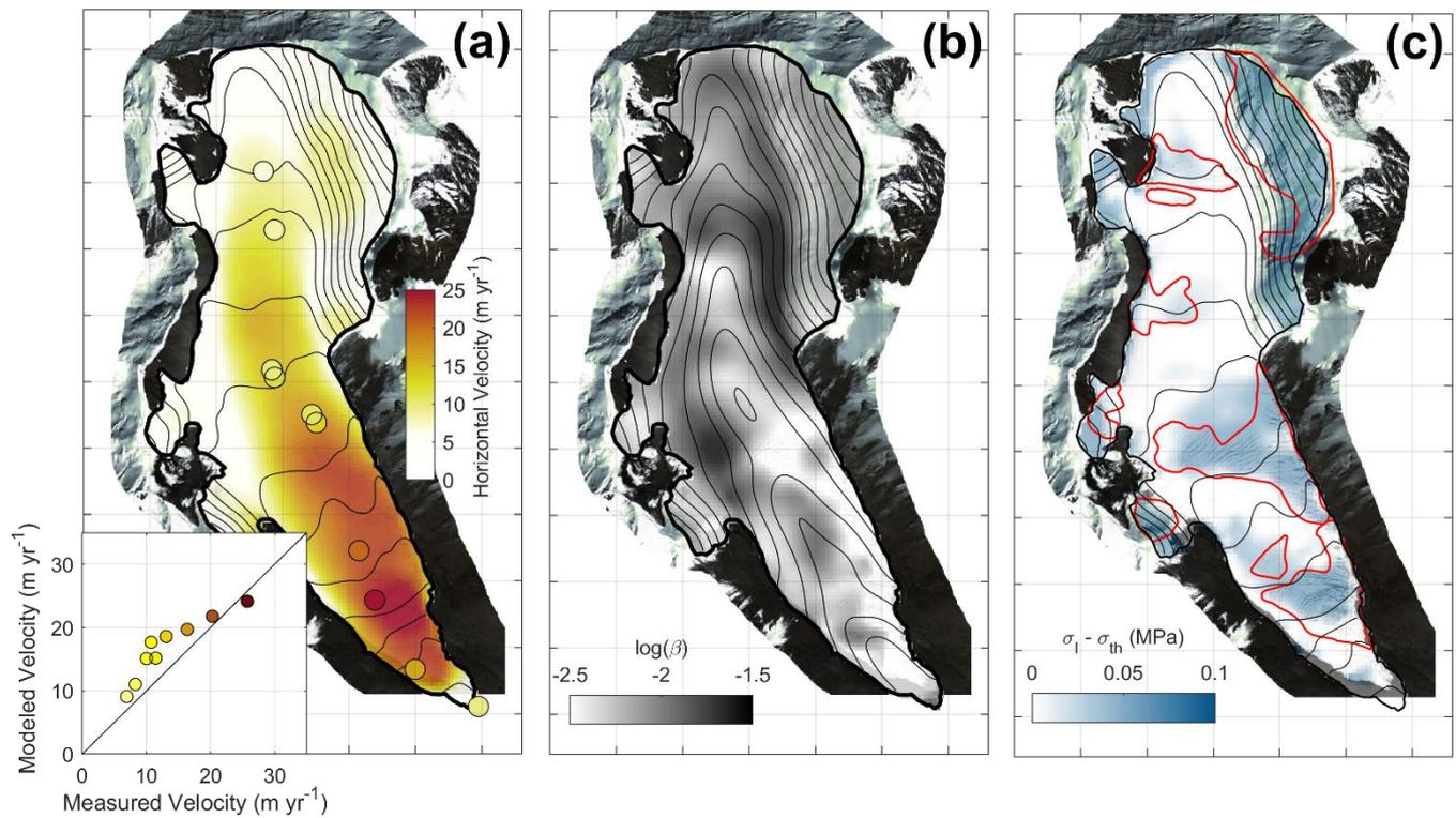
650 **Figure 7. (a) Steady state surface velocities compared with the measurements (coloured dots and inset). Contour lines are surface topography with 50 m intervals (b) Friction coefficient inferred from emergence velocities (assumed to be opposite of surface mass balance). Contour lines are bedrock topography with 50 m intervals (c) Modeled crevassed areas from maximal Cauchy stress anomaly (colour scale) compared with observations (red lines).**
