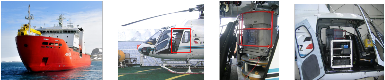
Figure 1. The helicopter gravity acquisition from RVIB Araon, 2015 - 2016. The photos from left to right are icebreaker RVIB Araon; Helicopter AS350 on board Araon loaded with gravimeter GT1A, the red box indicates the gravimeter; the GT1A gravimeter; GT1A's power electronics and GPS receiver.
