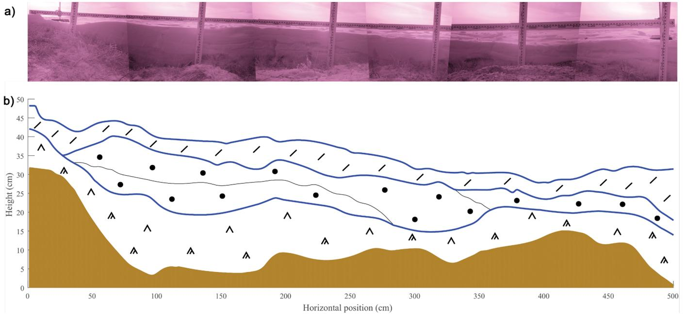
5 **Figure 2: a) Stitched NIR images of the trench face (Trench 10), b) Layer boundaries derived from NIR imagery, blue lines highlight boundaries between snow and air, surface snow and wind slab, as well as wind slab and depth hoar. The brown area is subnivean soil or vegetation. Symbols describe snow type following the classification of Fierz et al. (2009).**
