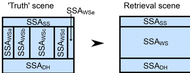
5 **Figure 3: Illustration of three-layer (SS: Surface Snow; WS: Wind Slab; DH: Depth Hoar) truth scene with spatial variability in Specific Surface Area of WS ( $SSA_{WSa}$  to  $SSA_{WSe}$ ) and the retrieval scene with horizontally uniform SSA. Spatial distribution in truth SSA given by observed spatial distribution at TVC over two winters (2013 and 2018).**
