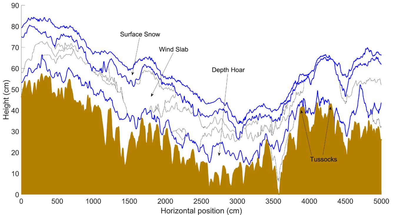
5 **Figure 6: Cross-section with vertical exaggeration of layer boundaries of individual stratigraphic layers in trench 4 (50 m). Blue lines highlight boundaries between snow and air, surface snow and wind slab, as well as wind slab and depth hoar. The brown area is subnivean soil or vegetation (two tussocks are labelled). Black lines show boundaries of individual layers aggregated within the wind slab and depth hoar layers.**
