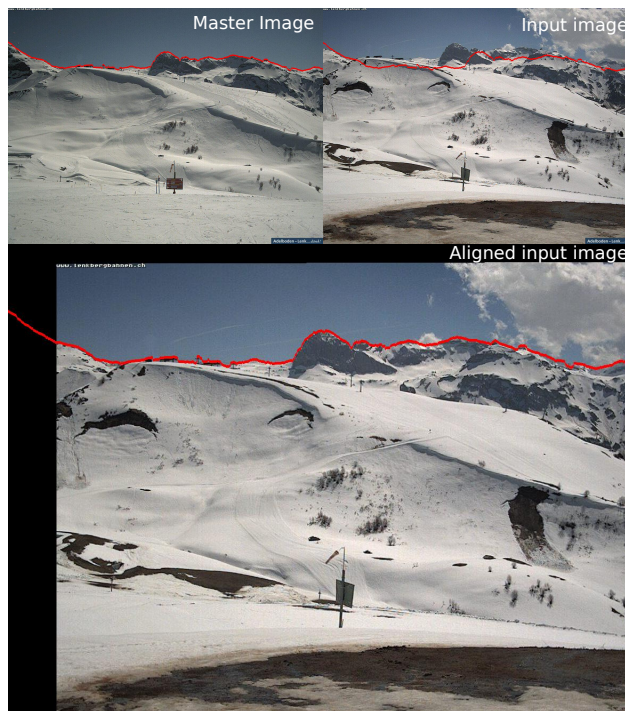
Figure 9. Example of an arbitrary input image that is aligned to a corresponding Master Image. The mountain silhouette extracted from the Master Image is shown in red.
