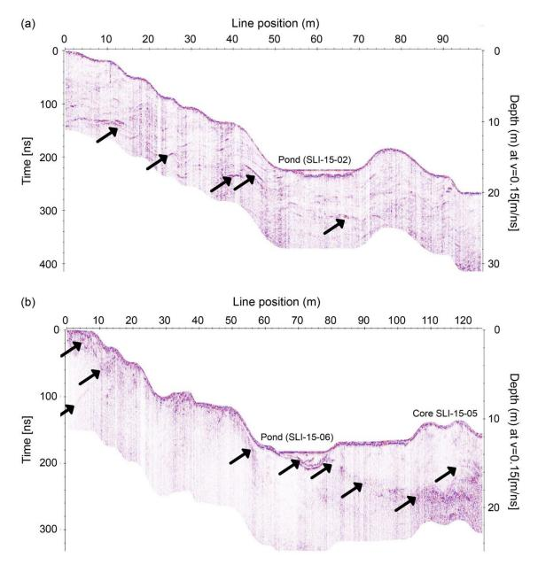
**Figure 11.** Processed 400 MHz ground-penetrating radar data from the transect down the rock glacier. a) Mid-rock-glacier line showing interpreted internal debris and a mid-rock-glacier pond (~50–70 m; site of ice core sample SLI-15-02 and -03). b) Part of the transect crossing the frozen pond (sample site SLI-15-06 and -07) near the lowest buried ice-core site (at 110 m; SLI-15-05). Arrows point to reflection events interpreted to correlate with internal debris layers.
