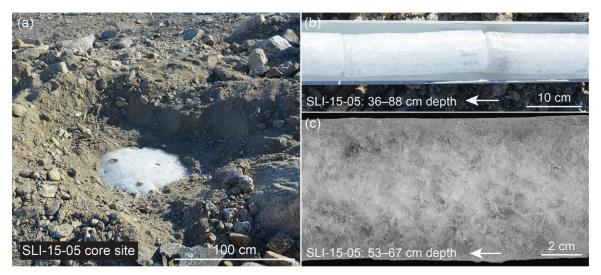
**Figure 4.** Buried ice core SLI-15-05. a) Excavation of ~30 cm of sand- and boulder-rich sediments above buried ice, exposing sharp contact between sediments and ice surface. b) Buried ice core pictured in the field, 36–88 cm depth below ice surface; up core is to the left (shown with arrow). c) Buried ice core (53–67 cm depth) after being cut vertically at NICL. At this depth, buried ice contained many gas inclusions and no sediments.
