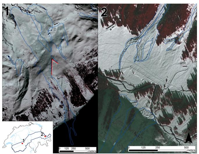
Figure 3: Examples of mapped avalanches in imagery optimized for brightly illuminated areas (1) and for regions with shaded areas (2). A deflection dam that worked well by changing the flow path of the avalanche is marked as red line in (1). (SPOT6 Data © Airbus DS 2018). Overlapping avalanches area is determined by interpretation of the flow direction from the topographic map
