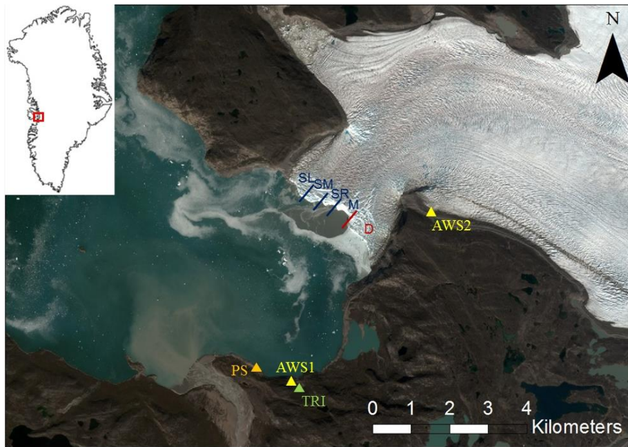
Figure 1: Overview of Ekip Sermia and measurement sites. The positions of the terrestrial radar interferometer (TRI), the pressure sensor (PS) and the two weather stations (AWS) are indicated by triangles. The deep and shallow calving front sectors are marked with red and blue lines. Background: Sentinel-2A scene from 3 August 2016 (from ESA Copernicus Science Hub: https://scihub.copernicus.eu ).
