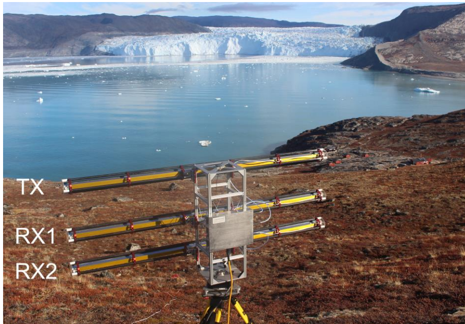
Figure 2: The terrestrial radar interferometer (TRI) located opposite of the front of Ekip Sermia at a distance of 4.5 km (image: M. Lüthi, 2016). The TRI has one transmitting (TX) and two receiving antennas (RX1, RX2).
