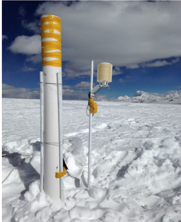
Figure 2. The equipment for collecting new snow samples from the surfaces of the seven studied TP glaciers.
