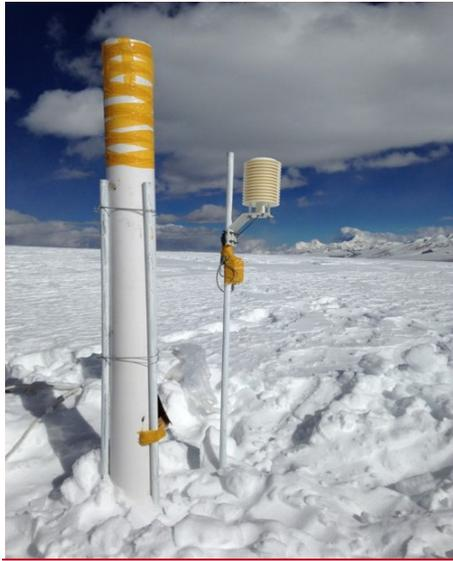
**Figure 2.** The equipment for collecting new snow samples in seven TP glaciers.
