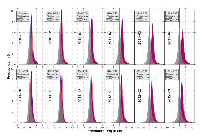
Figure 10. Histograms of freeboard for each month of the mission overlap period (in centimeters) for Envisat (red) and CryoSat-2 (blue) as well as the corresponding freeboard difference between both sensors (gray) for the Arctic. Furthermore, the average freeboard difference  $(\Delta Fb; Envisat minus CryoSat-2)$ , as well as the average freeboards for CryoSat-2 ( $Fb_{CS2}$ ) and Envisat ( $Fb_{ENV}$ ) are given in centimeters in the gray box for each month.
