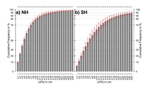
Figure 12. Cumulative frequencies of absolute freeboard differences (Envisat minus CryoSat-2) as shown in Figures 10 and 11 averaged over all months in the MOP. Data is presented for the northern hemisphere (a) as well as the southern hemisphere (b). Errorbars indicate  $\pm 1$  standard deviation. First bar covers the absolute freeboard difference range from [0cm:1cm[, second bin from [1cm:2cm[, and so on.
