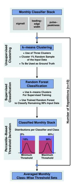
**Figure 1.** Flowchart visualizing the important sub steps of unsupervised clustering and supervised classification in order to derive the new surface-type thresholds from monthly stacks of sea-ice backscatter, leading-edge width and pulse peakiness.
