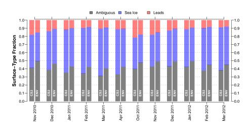
Figure 6. Time-series of surface-type fractions for the mission overlap period between CryoSat-2 (CS2) and Envisat (ENV) for the Arctic based on orbit-track (i.e., non gridded) data.
