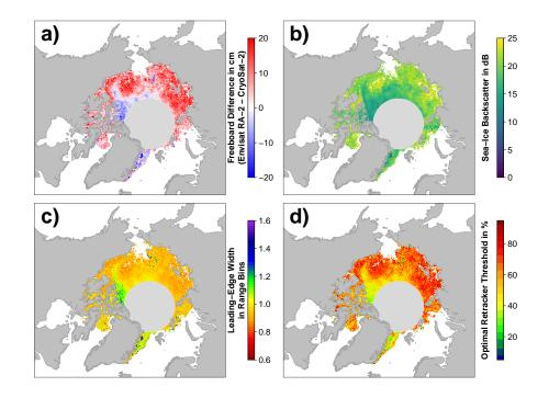
**Figure 2.** Exemplary visualizations of freeboard differences between Envisat and CryoSat-2 (a; in cm), Envisat sea-ice backscatter (b; in dB), Envisat leading-edge width (c; in range bins), and optimal retracker threshold (d; in %) for the Arctic in November 2011.
