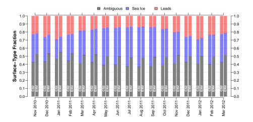
Figure 7. Time-series of surface-type fractions for the mission overlap period between CryoSat-2 (CS2) and Envisat (ENV) for the Antarctic based on orbit-track (i.e., non gridded) data.
