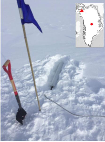
Figure 1: Photograph of Hydroinnova Snowfox™ cosmic ray neutron sensor (CRNS) exposed in firn trench on the first day of deployment. Inset shows the location of Summit Camp on the Greenland Ice Sheet, as denoted by the red circle. The red triangle shows the location of the THUL reference neutron monitor maintained by the University of Delaware Bartol Institute.
