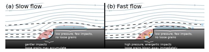
**Figure 15.** Conceptual model for air and particle flow over a snow-step in (a) slow-moving and (b) fast-moving air. Solid lines show idealized streamlines over the step, including two regions of detached flow (shaded in a). Dashed black lines show snowflake trajectories.
