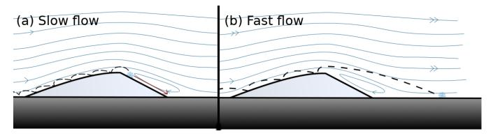
**Figure 14.** Conceptual model of grain transport over a dune in (a) slow-moving air and (b) fast-moving air. Solid blue lines are time-averaged streamlines, with boundary-layer fluctuations omitted for clarity. Dashed black line shows a grain trajectory. The arrow in (a) shows an avalanche path.
