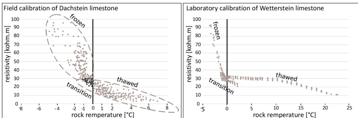
Figure 34: Comparison of small scale ERT (left) at MS-K and laboratory (right; Krautblatter et al. 2010) calibration measurements.
