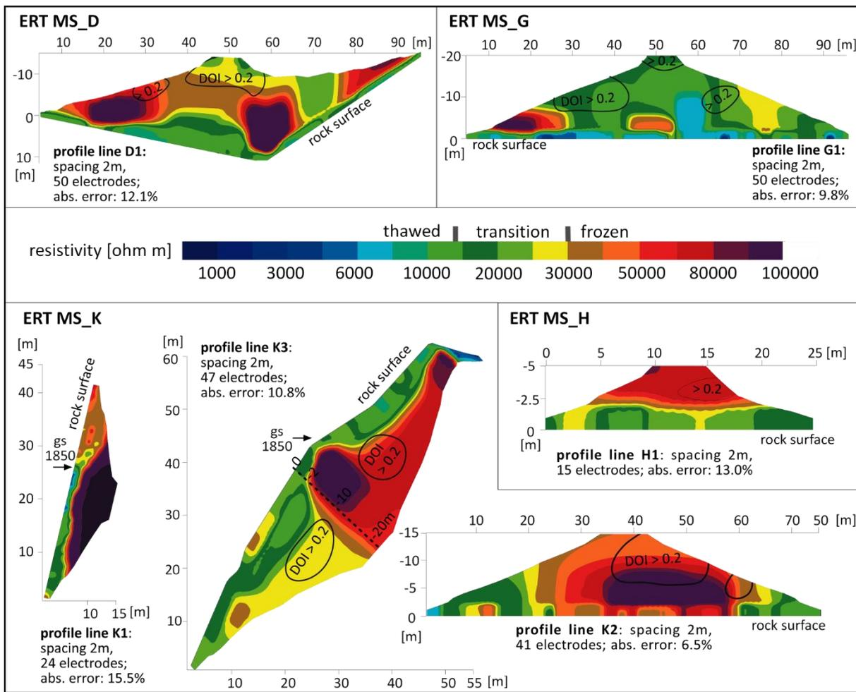
Figure 6: ERT results at **MSMS--D** (measurement site Dirndln), **MSMS--G** (Gjaidstein), **MS-K** (Koppenkarstein) and **MS--H** (Hunerkogel). gs 1850 = glacier surface at c. 1850
