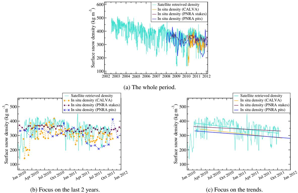
**Figure 6.** Time series of the snow density near the surface at Dome C, Antarctica, retrieved from AMSR-E passive microwave observations and measured in the field (3 different datasets) from 18 June 2002 to 4 October 2011 (a). The graph (b) focuses on the last two years and the graph (c) on the trends during the last two years.
