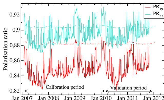
**Figure 3.** Time series of modelled (lines) and observed (dots) polarisation ratios at 19 and 37 GHz ( $PR_{19}$  and  $PR_{37}$ ) at Dome C, Antarctica, during the calibration period (2007–2009) and the validation period (2010–2011).
