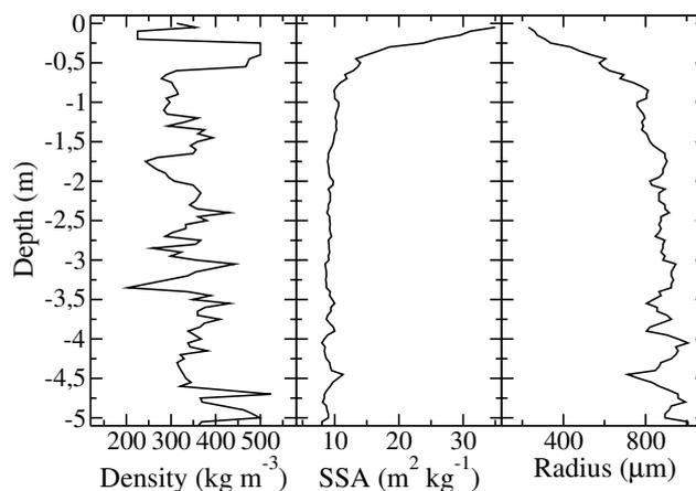
**Figure 1.** The profiles of snow density, SSA and DMRT-ML radius at Dome C, Antarctica. DMRT-ML radius is derived from SSA measurements and is the input of the model (Sec. 2.2.4 and Eq. 1 and 2).
