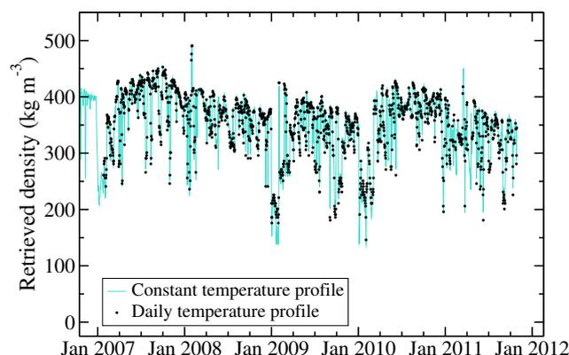
**Figure 9.** Time series of the snow density near the surface  $\rho_{\text{sat}}$  at Dome C, Antarctica, retrieved from AMSR-E passive microwave observations and covering the period from 1 December 2006 to 4 October 2011: (black dots) using the temperature profile of each day and (solid grey line) using a temperature profile constant in time.
