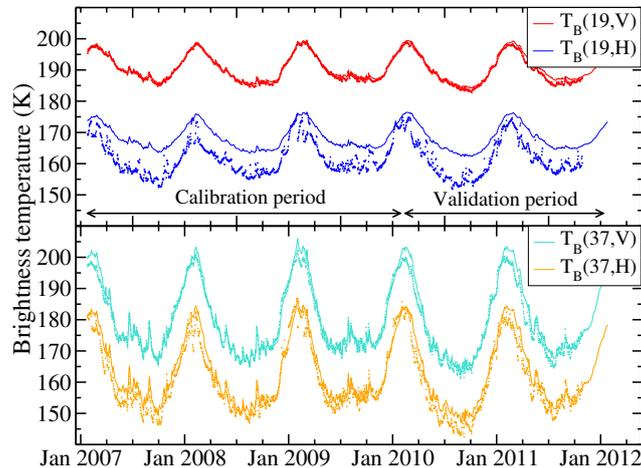
**Figure 2.** Time series of modelled (lines) and observed (dots) brightness temperatures, at 19 and 37 GHz and at vertical and horizontal polarisations ( $T_B(19, V)$ ,  $T_B(19, H)$ ,  $T_B(37, V)$ ,  $T_B(37, H)$ ) at Dome C, Antarctica, during the calibration period (2007–2009) and the validation period (2010–2011).
