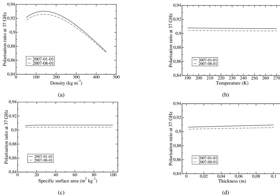
**Figure 4.**  $PR_{37}$  variations caused by changes in snow properties of the top layer: (a) density, (b) temperature, (c) SSA and (d) thickness. The two different dates correspond to typical winter and summer temperature profiles.
