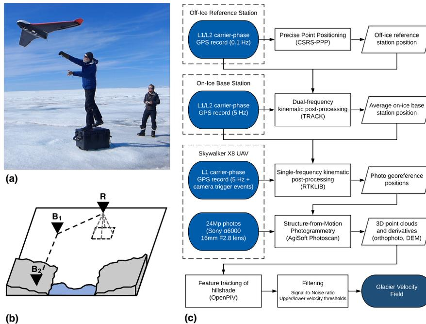
**Figure 2.** The method used in this study: (a) Launching the Skywalker X8 on the ice sheet; (b) cartoon ~~showing process~~ visualising the relationship of kinematic GPS corrections between the UAV rover (R), on-ice launch site base station (B<sub>1</sub>), and the off-ice reference station (B<sub>2</sub>); and (c) flowchart showing the workflow used in this study to derive photogrammetry products and velocity fields at the inland study site.
