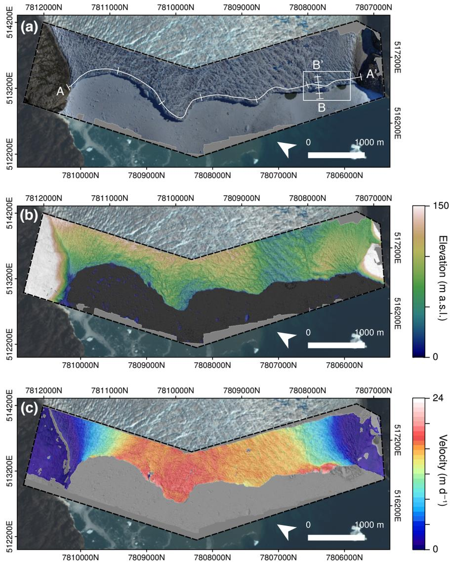
**Figure 3.** Example data output from calving front. (a) 0.15 m orthophoto, collected 10:15 12<sup>th</sup> July 2017. (b) 0.2 m DEM from same flight. (c) 6-hour ~~seperation~~ separation velocity field ( $\sigma_v = \pm 0.69$  m) from 16:15–22:15 on the 12<sup>th</sup> July. Transects in (a) refer to Figure 4. Box refers to location of Figure 5
