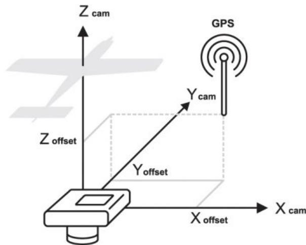
**Figure 1** | GPS/INS offset coordinate system. Figure taken from Photoscan documentation (Agisoft, 2018).
