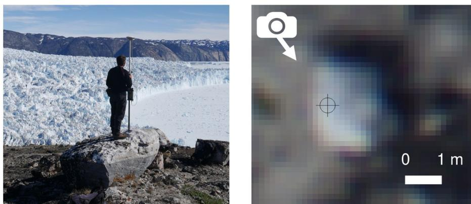
**Figure 2** | Example of validation GCP collection (left) and comparison against orthophoto (right) at calving front. Direction of photograph origin shown by white marker.
