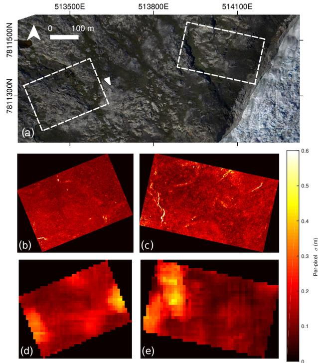
**Figure 6.** Error assessment at the calving front: (a) location of two validation sites at the calving front shown on UAV-derived orthophoto; (b-c) standard deviation in Z axis derived from DEMs (d-e) standard deviation in XY axes derived from horizontal displacement fields.
