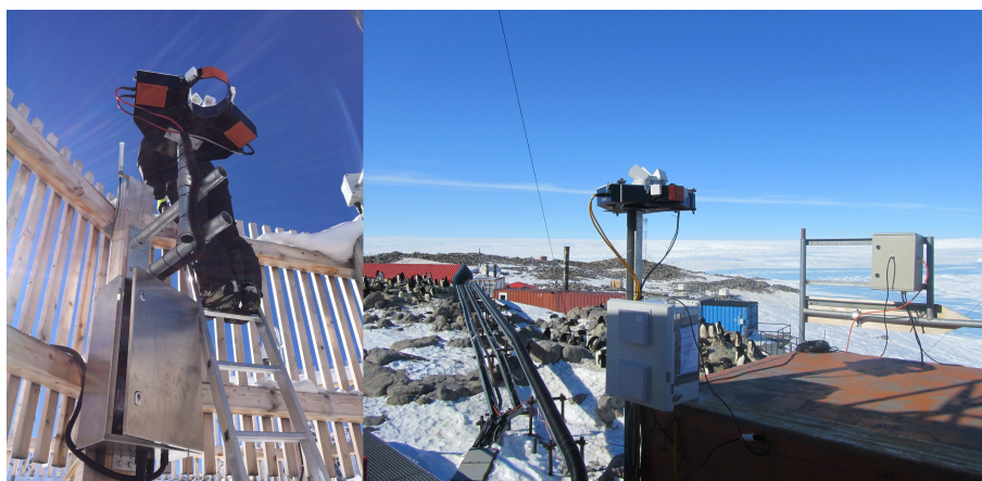
Figure 1. Experimental set-up conditions of the MASC in a DFIR near Davos (left) and on top of a container at DDU (right).
