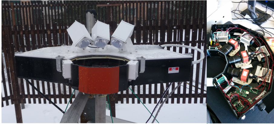
Figure 1. Left: side-view of the MASC with the three flash lamps in white on top, the two detectors as white boxes on the side of the metal ring (in black and red in front). Right: top view of the inside of the MASC, with the three cameras clearly visible.
