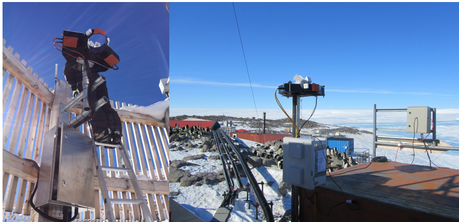
Figure 2. Experimental set-up conditions of the MASC in a DFIR near Davos (left) and on top of a container at Dumont d'Urville (right).
