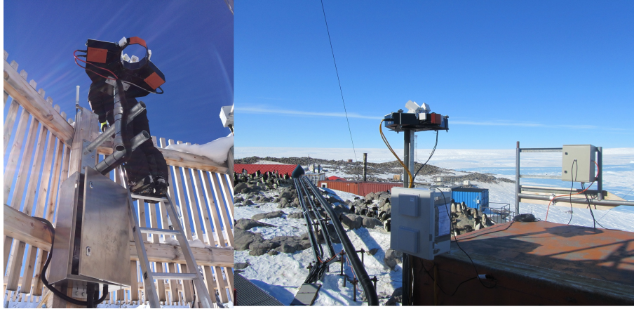
Figure 2. Experimental set-up conditions of the MASC in a DFIR near Davos (left) and on top of a container at DDU Dumont d'Urville (right).
