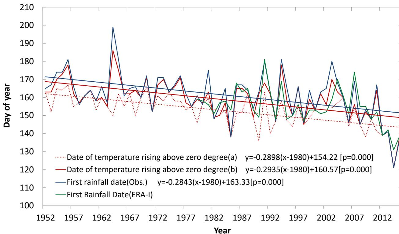
**Figure 7: Timing of air temperature exceeding 0°C for the first time and the timing of first rainfall in spring at WSO AP site, 1952-2015. The red dashed line (a) corresponds to the first instance of air temperature above 0°C. The red solid line (b) indicates the first warming event continuing for at least 4 days. P denotes significance value of the linear trend.**
