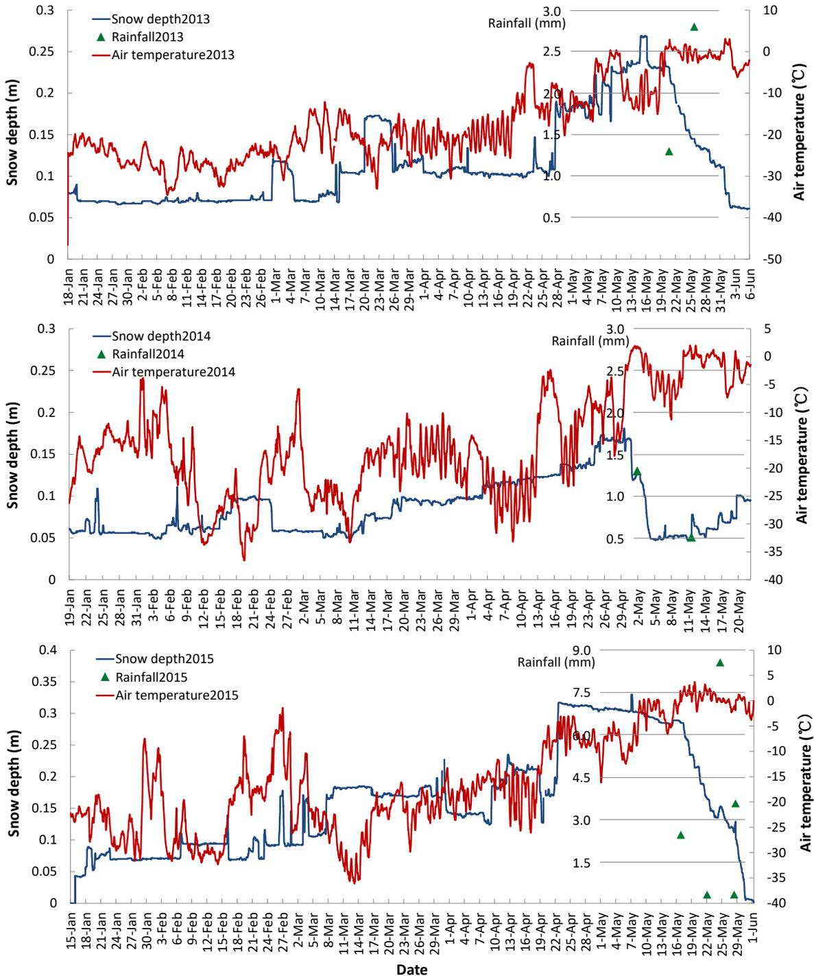
**Figure 1:** Rainfall and variations in air temperature and snow depth recorded near Pt. Barrow, Alaska. The data was observed at MB site on Chukchi Sea landfast ice between January and June in 2013, 2014 and 2015. Amount (mm-we) and timing of rainfall are indicated by blue triangles.
