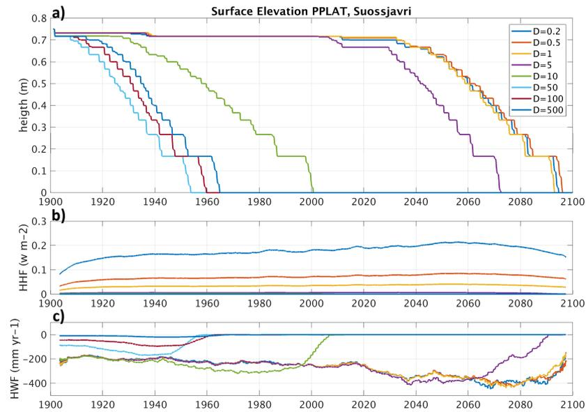
**Figure 11: Surface elevation of PPLAT at Suossjavri, Northern Norway (a) for different values of distance parameter ( $D$ ) between the two interacting tiles, and corresponding horizontal heat flux (HHF; b), and horizontal water flux (HWF; c). Note that the area of PPLAT is different (larger) here than in the standard simulations (Fig. 7), giving a different evolution for the same ( $D=10$ ) distance parameter.**
