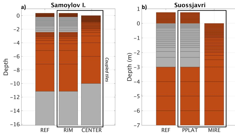
**Figure A1: Vertical resolution and at Samoylov Island (a) and Suossjavri (b). Gray colours indicate layers initialized with excess ice. Excess ice initiated in bottom layer at Samoylov Island is used to adjust the rim height ( $e_r$ ) independently of near-surface excess ice.**
