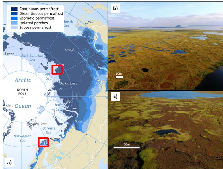
**Figure 1: a) Location of the two test sites on top of the map of permafrost distribution in the Arctic (Brown et al. 1998). b) example of low-centered polygons on Samoylov Island, Northern Siberia (Photo: Sebastian Zubrzycki). c) Example of peat plateau near Suossjavri, Northern Norway (Photo: Sebastian Westermann). The two sites are located in the continuous and sporadic permafrost zones, respectively.**
