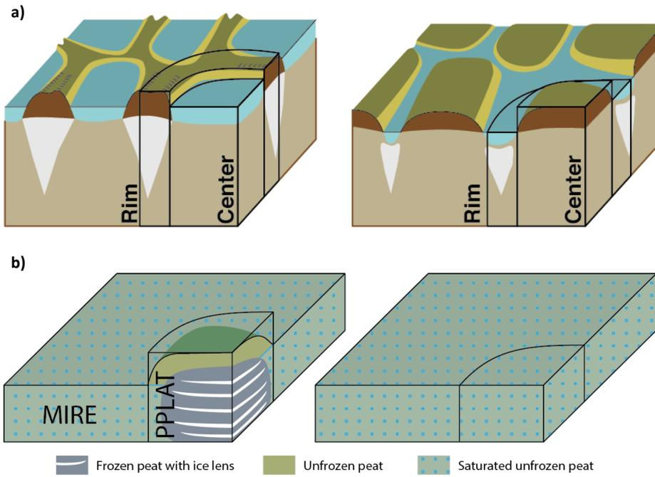
**Figure 2: a) Schematic presentation of undegraded, low-centred polygon (left) and degraded, high-centred polygons (right) with corresponding tiles used in this study (adapted from Liljedahl et al. 2016). b) Schematic presentation of peat plateau in a surrounding mire (left), and the mire after the peat plateau has degraded (right), with corresponding tiles.**
