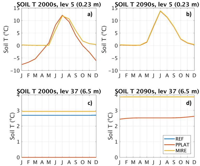
**Figure 8: Average annual temperature cycle during first (a, c) and last (b, d) decade of 21<sup>st</sup> century at Suissjavri, Northern Norway, in the 5<sup>th</sup> model layer (a, b; 0.23 m below surface) and the 37<sup>th</sup> model layer (c, d; 6.5 m below reference height). See layer depths in Fig. A1b.**
