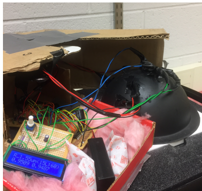
Figure 2. Near-Infrared Emitting and Reflectance-Monitoring Dome (NERD) schematic (top) and photographs (bottom). The photograph on the bottom right shows the (radial) placement of photodiodes and LEDs (toward the center) within the dome.
