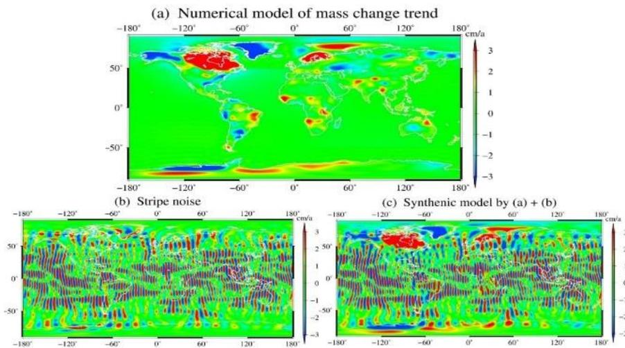
Figure 1. (a) The numerical model of mass change trend, (b) the stripe noise model; (c) synthetic model by (a) + (b).
