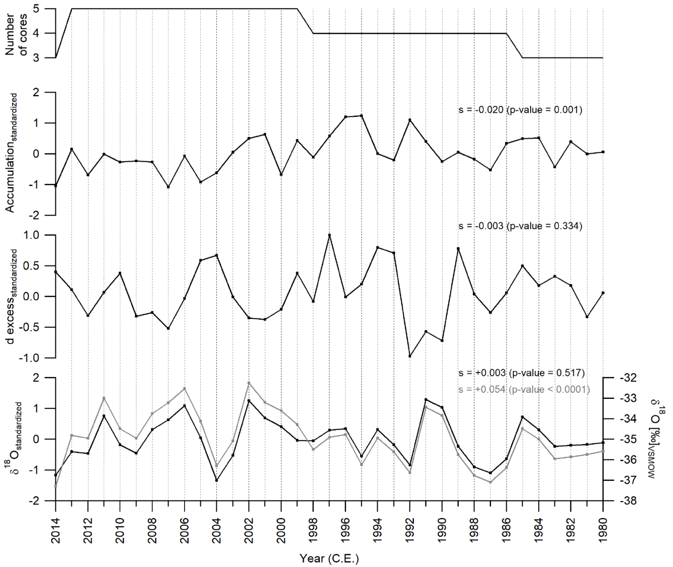
Figure 8: Composite records of mean annual \delta^{18}\text{O} , d excess and snow accumulation in the UG region for the period 1980-2014 derived from standardized data (black; excluding firn core GUPA-1). Sen slopes (s) and p-values (p) are given for each record. For \delta^{18}\text{O} , the composite record derived from non-standardized annually averaged data (grey) is also displayed as it exhibits a
