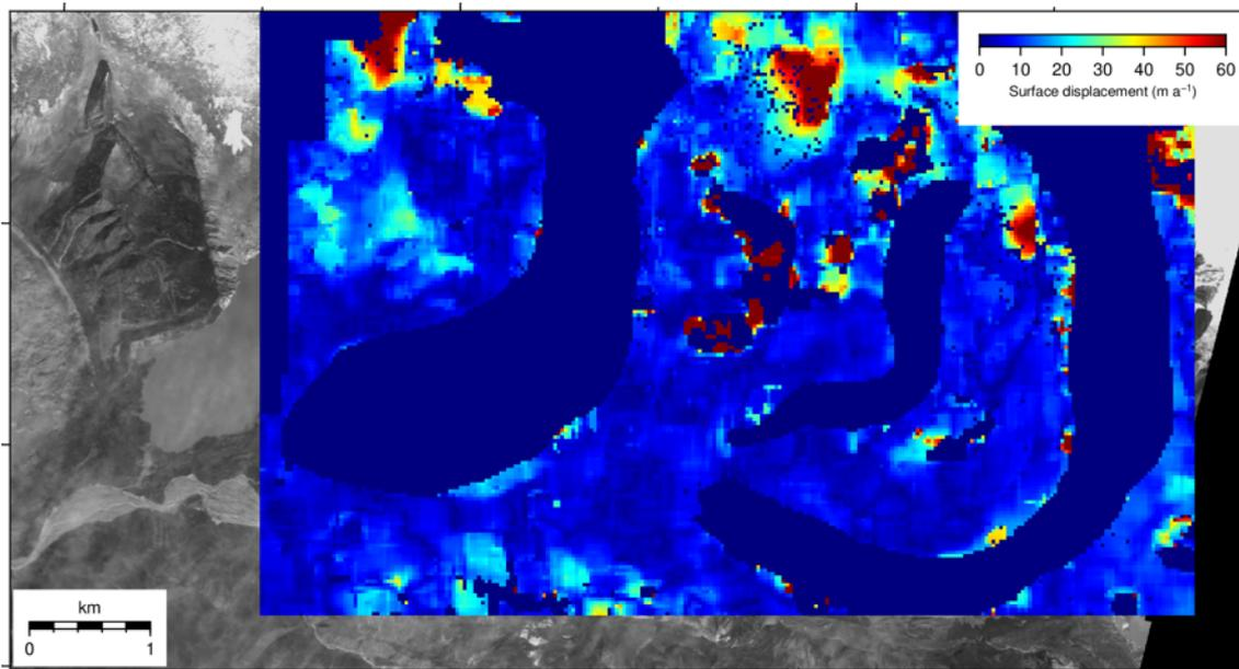
**Figure R12:** Surface displacements on ice-free terrain derived from image pair on 3 February 2006 and 30 January 2007.
