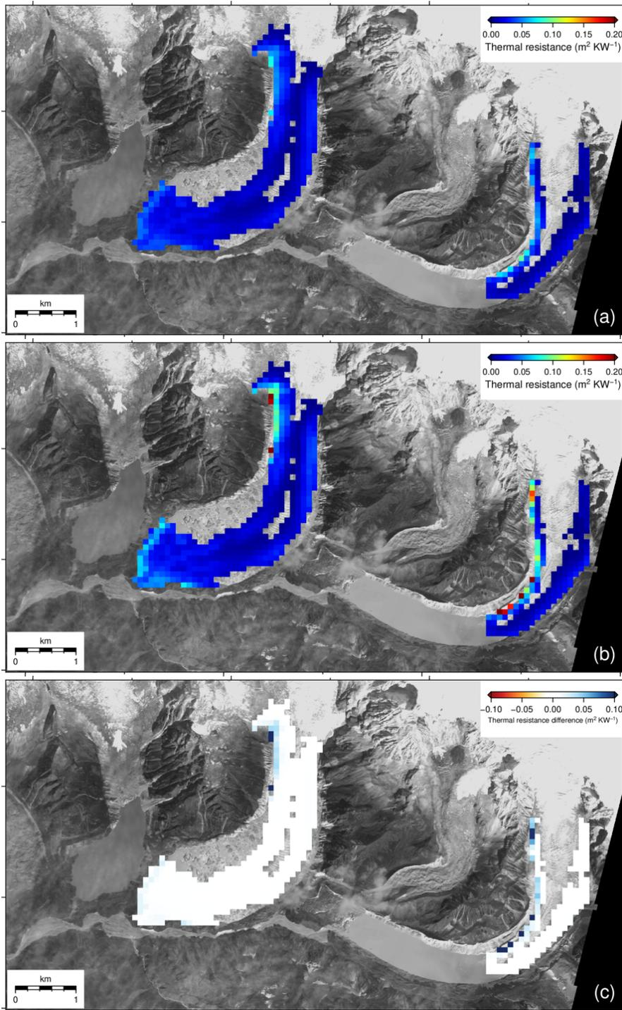
**Figure R5:** Spatial distribution of thermal resistance calculated (a) from only net radiation, (b) from net radiation + sensible heat and (c) difference of thermal resistance calculated by the two methods.
