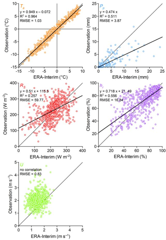
Figure R7: Scatter plot of air temperature, precipitation, solar radiation, relative humidity and wind speed between ERA-Interim reanalysis and observational data for 2002–2004.
